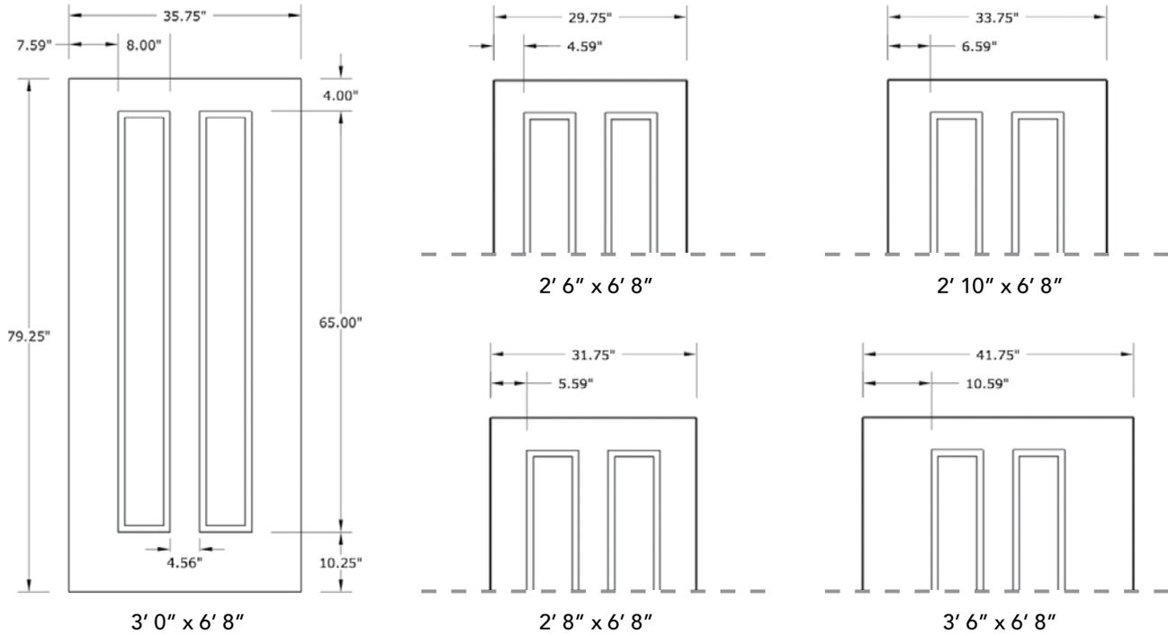
NOTE: BY REQUEST, DOOR HEIGHT COMES IN VARYING DIMENSIONS TO A MINIMUM OF 79". EXCESS WILL BE TAKEN FROM BOTTOM RAIL. ALL OTHER DIMENSIONS WILL REMAIN THE SAME.
